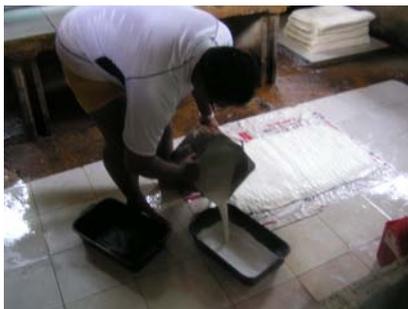
Between Mr. T and the resident farmers, they showed how the whole process works. The rubber curing process involves having a large tub filled with the white rubber
